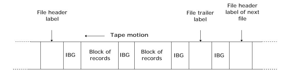
Illustrates the concepts of multiple blocks of records forming a file that is separated from other files by a <u>file header label</u> in the beginning and a <u>file trailer label</u> at the end of the file
