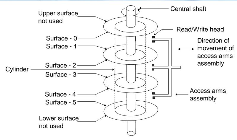
No. of disk platters = 4, No. of usable surfaces = 6. A set of corresponding tracks on all the 6 surfaces is called a cylinder.
