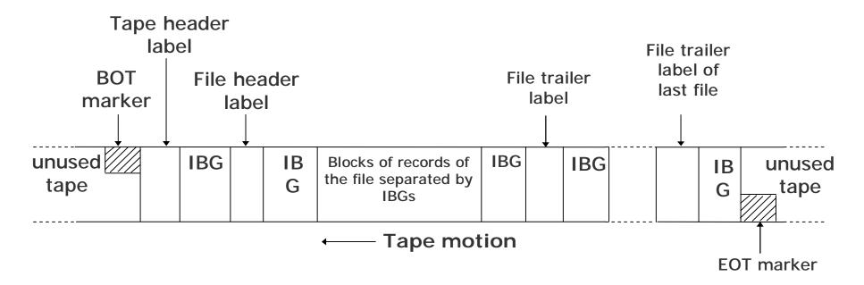
Illustrates the concepts of Beginning of Tape (BoT) and End of Tape (EoT) markers, and tape header label
