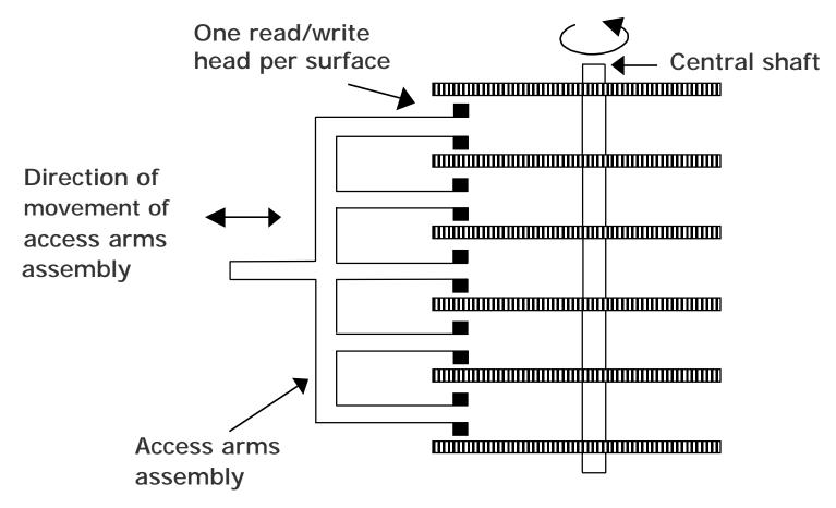
Vertical cross section of a disk system. There is one read/write head per recording surface
